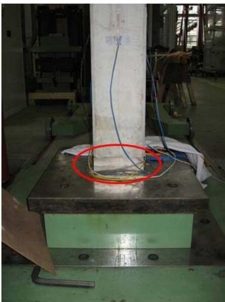
Fig. 14: Conditions of column S5 under a compressive strain of 4.5‰, first signs of scaling bottom left (encircled)
